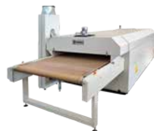
Exhaust fumes and outlet cooling hood
