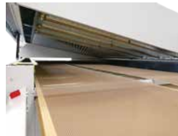
Infrared Lamps and upper section opening
