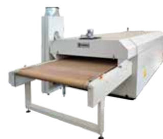
Exhaust fumes and outlet cooling hood
